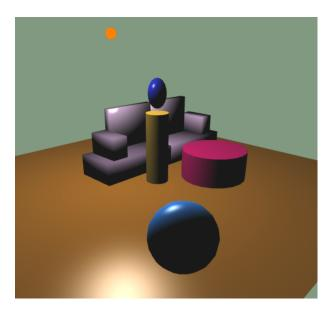
Then, the scene was enhanced with Phong per-fragment shaders to create a global illumination effect. The orange sphere represents the light and can be controlled using the z, x, c, v, b, and n keys.
