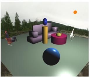
Finally, more complex shape models from outside sources were imported into the project. The teapot was shaded in a similar manner to the furniture, while the roosters are texture mapped. In addition, the teapot is animated so that it rotates on the coffee table. An environment cube mapping was used to create the background and make one of the roosters reflective.
